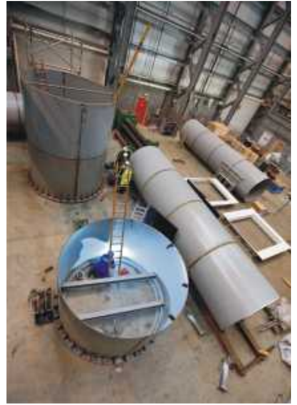
Welder/fabricator Andy Paterson welding one of the rings that will form the stack
