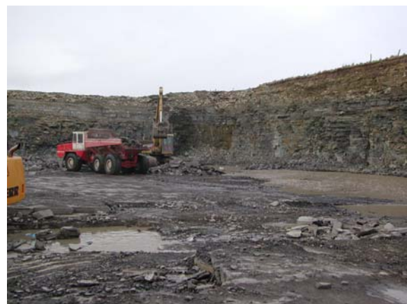
Excavation of Caithness flagstone
