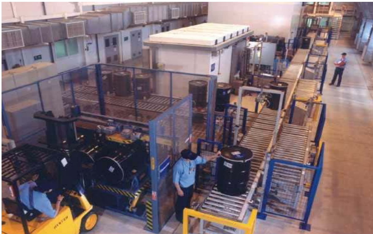
Photograph of the interior of the Dounreay Waste Receipt, Assay, Characterisation & Supercompaction facility, showing inspection of LLW drums.
