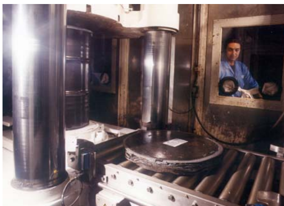
Photograph of the interior of the Downreay Waste Receipt, Assay, Characterisation & Supercompaction facility, showing compaction of LLW drums into thin “pucks” (left), and filling of a HHISO container with compacted LLW drums (right).
