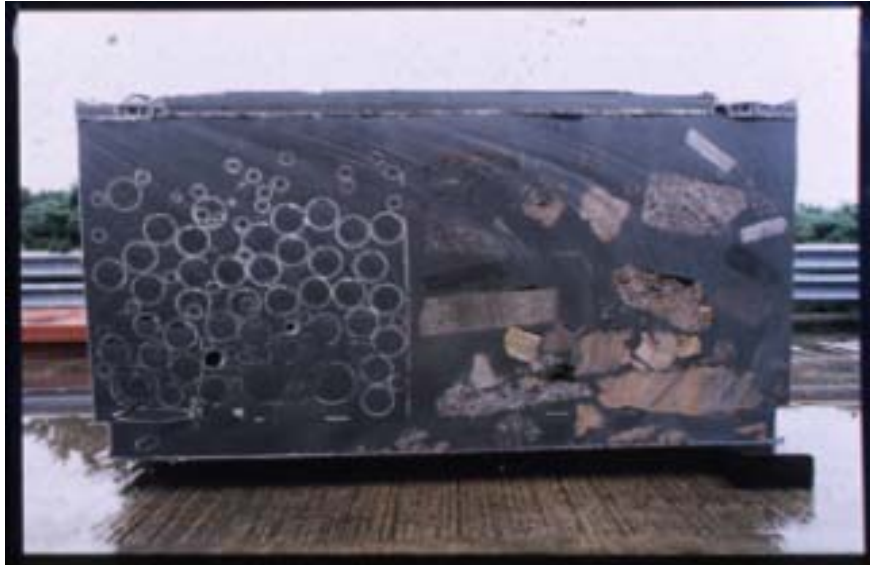
Photograph showing a cutaway view of a filled and grouted HHISO container (from the existing National LLW disposal facility near the village of Drigg in Cumbria). Note that this container did not contain actual radioactive waste, and the grouting work was performed for demonstration purposes.
