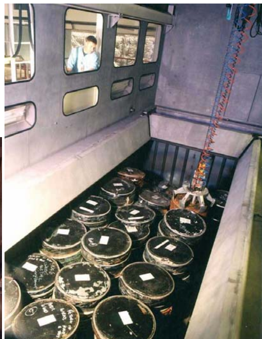
Photograph of the interior of the Downreay Waste Receipt, Assay, Characterisation & Supercompaction facility, showing compaction of LLW drums into thin “pucks” (left), and filling of a HHISO container with compacted LLW drums (right).
