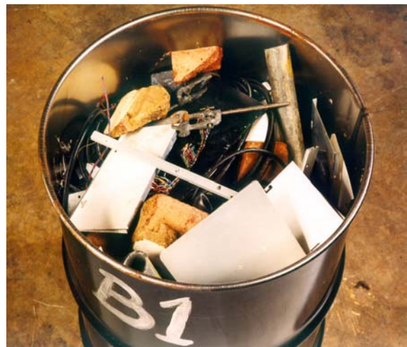
Photograph showing typical contents of a drum of Dounreay LLW.
