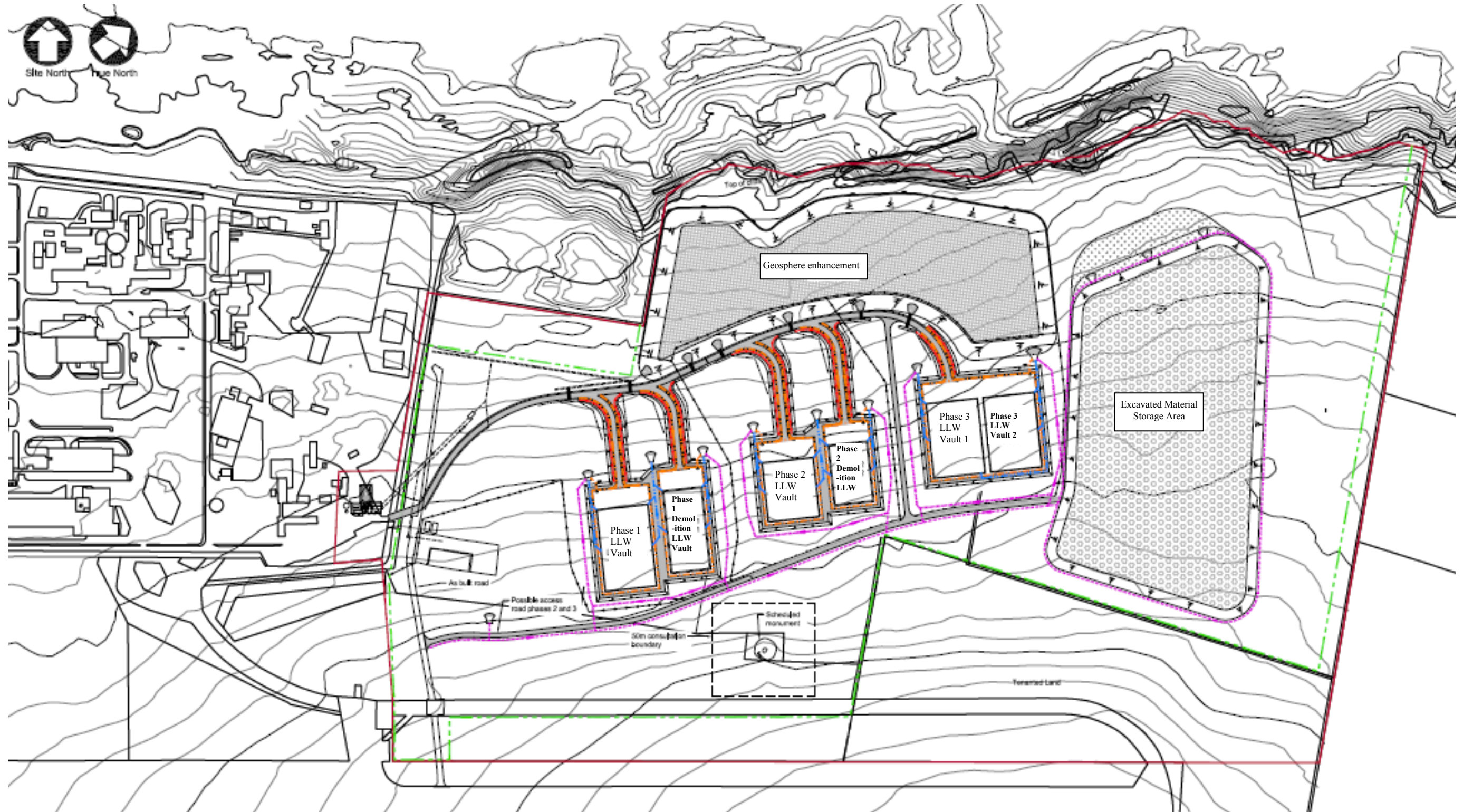
Figure 2 Refined layout plan for the New LLW Facilities currently being considered for the scheme design [extracted from Drawing Z266590]. Red line shows site development boundary. Note that the drawing is orientated to Dounreay site grid north.
