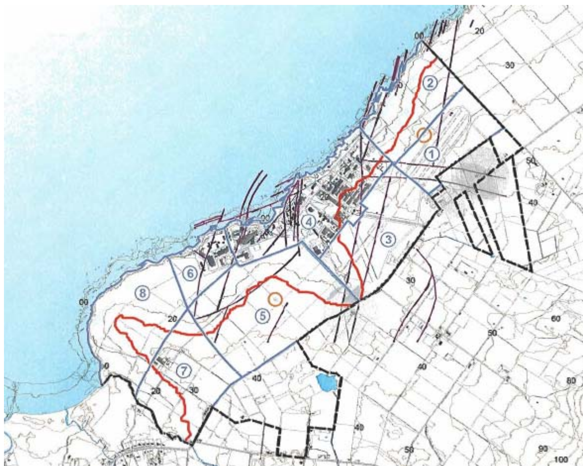
Figure 2. Areas (circled numbers 1 to 8) on UKAEA-owned land at Dounreay considered in selecting sites for the proposed new LLW disposal facilities. Also shown is the red line used as a siting objective to avoid areas that could be affected by future sea-level rise and coastal erosion over 10,000 years.
