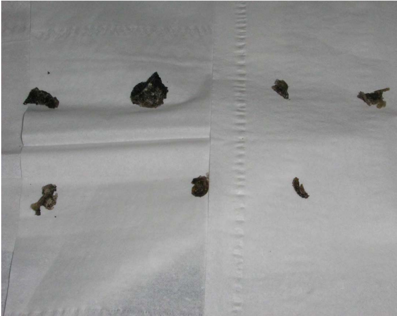
Figure 5 - Pieces of plastic separated from the active area. Each piece contained ^{137}\text{Cs} and ^{241}\text{Am}
