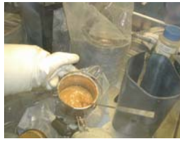
Figure 8: Actual Ammonium DiUranate (ADU) Floc
