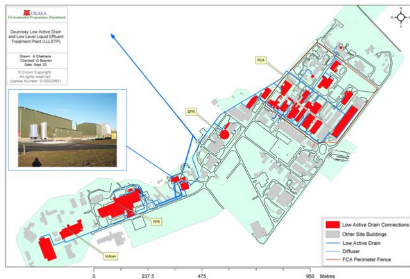
Figure 45: Low Active Drain System & Discharge Points
