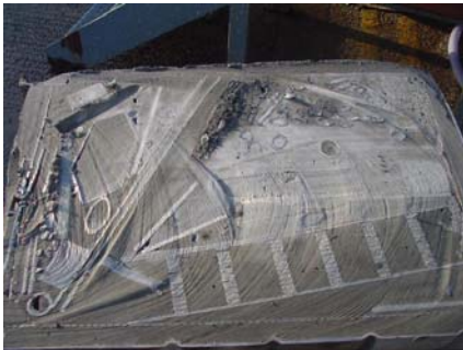
Figure 9: Sectioned Solid RHILW 500l Drum
